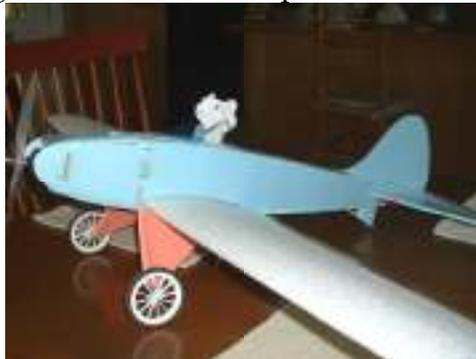
The Plane is my own design based on the universal fuse plan located on the FoamFly.com website. The fuse uses fanfold foam cut with interlocking joints. The designer refers to it as the zipper method. The parts join easily and make alignment much simpler. On the website he has several planes that he has designed around this fuse. The wing is a 36" E-205 EPP foam wing cut using the clubs CNC machine. All up weight with 2 cell lipo was 16oz.
