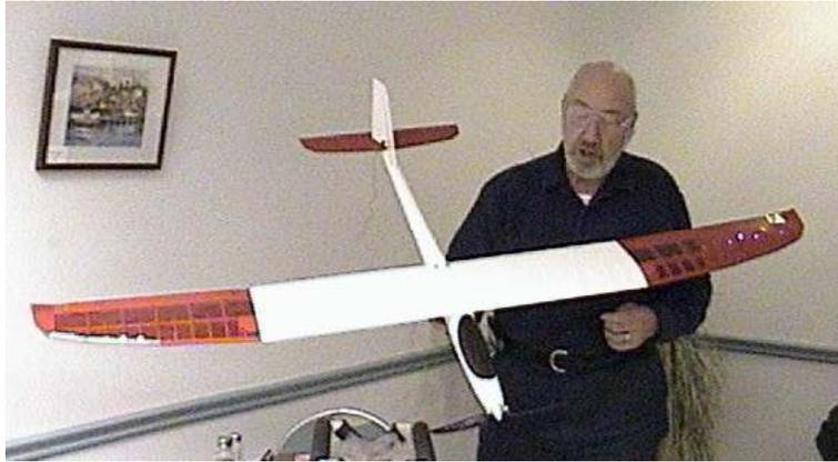
The wing has ailerons on the outer panel and they are finished and hinged. The wings have servo bays installed and the wiring is installed and ready for the servos. This is one of the finest examples of the excellent work that is done in the Czech Republic.
