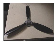
The task was to make a scale prop with 3 blades that were exactly the same for my current warbird project. I decided to make a glass mold and cast them in resin. The major difference in making the blades was that there isn't a nice place to divide the mold halves. The blade "plug" was carved from High Density Urethane foam, sanded, and filled, and sanded again. The same as the DLG "plug" that Jeff has made since.
