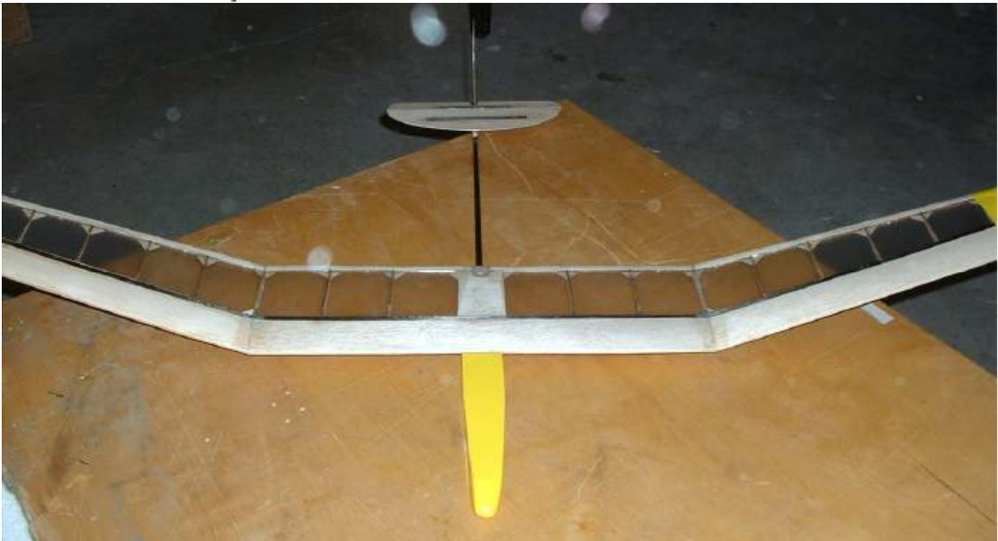
On my previous gambler the trailing edge bent up after a number of hard launches. Used gussets at each rib. Seemed to stiffen the wing torsionally quite a bit. So may prevent this problem with minimal weight addition. Glassed the polyhedral joints as well. Also found cutting the kevlar cleanly
