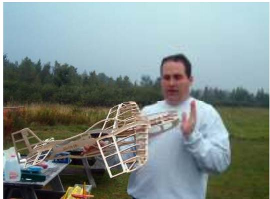
These kits provide all of the wood you will need to build your Electric Profile Airplane along with laser cut control horns, and carbon fiber push-rods. You'll need to provide all of your electronics (RX, Servos, Motor, Prop, Speed Controller, and Battery)."
