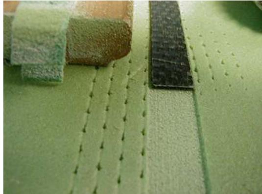
The sanding tool was used to make a slot. In this case reviewing the pictures you can see the slot is not deep enough. Question then becomes more sanding or more layers of paper to make the depth greater.
